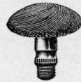
Figure 14 Steel wire brush to be used with flannel patches on shotgun rod
